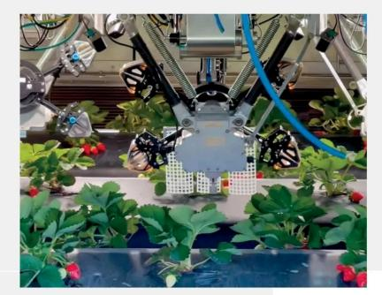
Gary Wishnatzki, the owner of Plant Citybased Wish Farms, utilizes an autonomous harvester equipped with Al-enabled robots to pick ripe strawberries.
